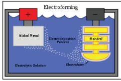
During the plating process, the mandrel acts as the cathode while the source of the electroform material is the anode. Controlling the time, current and current density in the plating tank will control the thickness of the electroform. Constant monitoring of the chemistry within the tank results in a more precise component.
