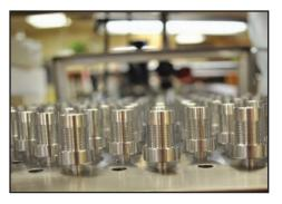
The mandrel is the base machined component, typically made from Aluminum 6061T or stainless steel, which defines the internal geometry of an electroform. In component manufacturing, it is typically more difficult to hold internal dimension to tight tolerances than external dimensions. Since electroforms are based on the machining tolerances of the external mandrel geometry, the internal dimensions are precise.
