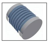
After the plating process, the mandrel will need to be removed from the assembly. For an aluminum mandrel, this is accomplished by exposing a portion of the mandrel; for example, the mandrel is made slightly longer than required when manufacturing an electroformed bellows. The ends are trimmed after plating to the desired length to expose the mandrel.
